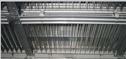
PSP-Ionizer blades of stainless steel
